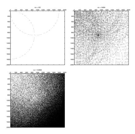
**Figure 1.** The points *added* in the second, third and fifth generation of the iteration from the implementation of the Bobylev-Cercignani method. In the fourth generation 1862118 of the in all 2 million points are added, and with the dot size used in the other plots, the square would be completely filled. The plots show one quadrant, with the origin in the upper left corner.
