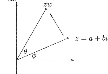
$$\begin{aligned} z &= a + bi \\ &= r(\cos \phi + i \sin \phi) \\ w &= \cos \theta + i \sin \theta \\ zw &= r(\cos(\theta + \phi) + i \sin(\theta + \phi)) \end{aligned}$$
