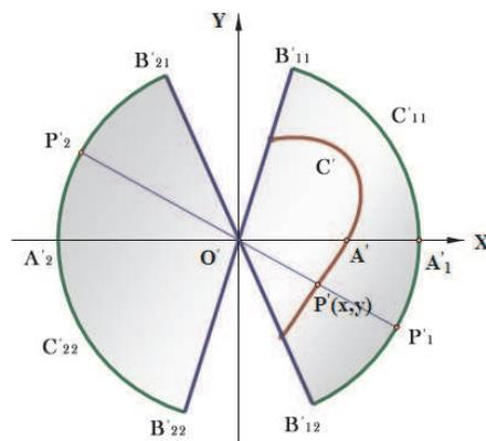
顯然，對頂錐面展平前後，有向弧  $\widehat{A'_1P'_1} =$  有向弧  $\widehat{A_1P_1}$ ,  $O'P' = OP = \rho$ ,  $|O'A'_1| = |OA_1|$ , 所以  $\angle A'_1O'P'_1 =$  有向弧  $\widehat{A'_1P'_1} \div |O'A'_1| =$  有向弧  $\widehat{A_1P_1} \div |OA_1| = (|OA_1| \sin \beta \cdot \varphi) \div |OA_1| = \sin \beta \cdot \varphi$ ,  $O'P' = \frac{h}{\cos \alpha \cos \beta - \sin \alpha \sin \beta \sin \varphi}$ .
